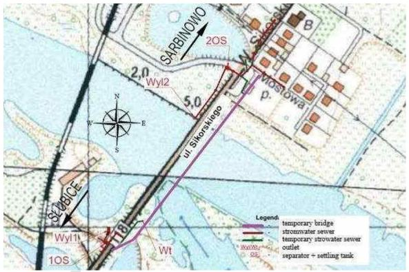
Fig. 1 Diagram of target and temporary stormwater drainage system
